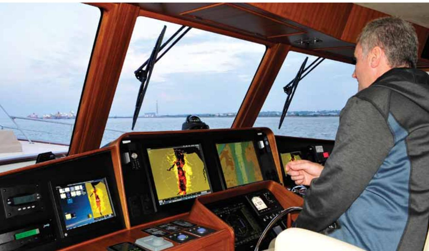
weight and reducing the size of wire bundles. In addition, a host of systems can be easily and routinely monitored from aboard the boat and remotely. An SMS text feature also allows the system to send important alerts, such as high water in the bilge, low voltage and smoke, to multiple users.
