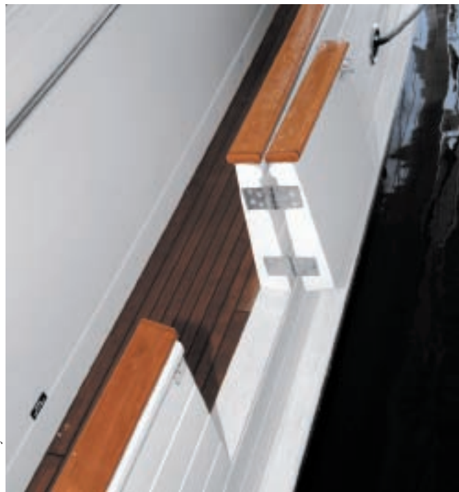
Top: Side deck gates now open into the side deck, unlike the original side door (above), which could sometimes be blocked by pilings or docks, by opening out making access difficult.
