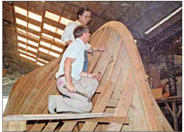
Left —Building the deck plug for the first Fleming, a 50-footer (15.2m) designed by Larry Drake, at the Tung Hwa Industrial Company, in Taiwan. Right —Fleming and Frank Ling hammer a ceremonial last nail into the hull plug frame for the same boat. Fleming had the tooling made for a 55' (16.8m) hull that was dammed-off to produce the 50' model.
