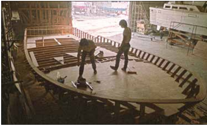
Left —Building the deck plug for the first Fleming, a 50-footer (15.2m) designed by Larry Drake, at the Tung Hwa Industrial Company, in Taiwan. Right —Fleming and Frank Ling hammer a ceremonial last nail into the hull plug frame for the same boat. Fleming had the tooling made for a 55' (16.8m) hull that was dammed-off to produce the 50' model.
