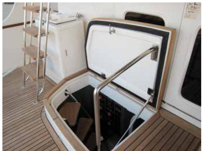
Engine room access with folding safety rail
