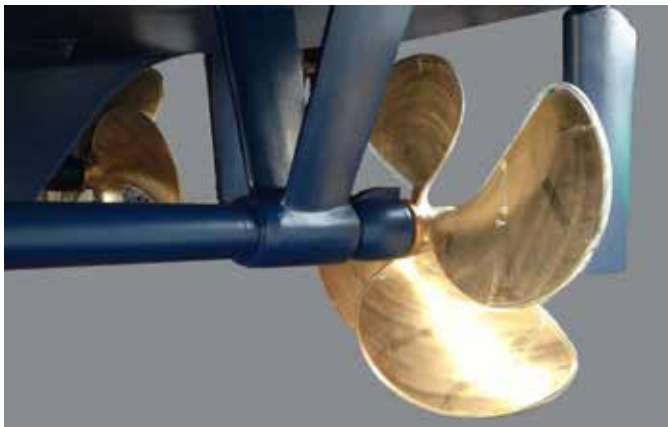
Seatorque shaft tube with rope cutter
