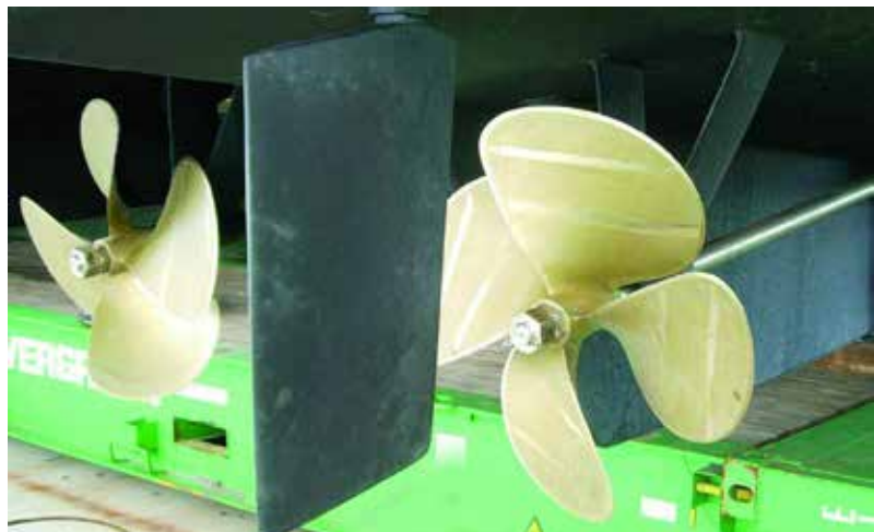
Deep full-length keel protects the running gear
