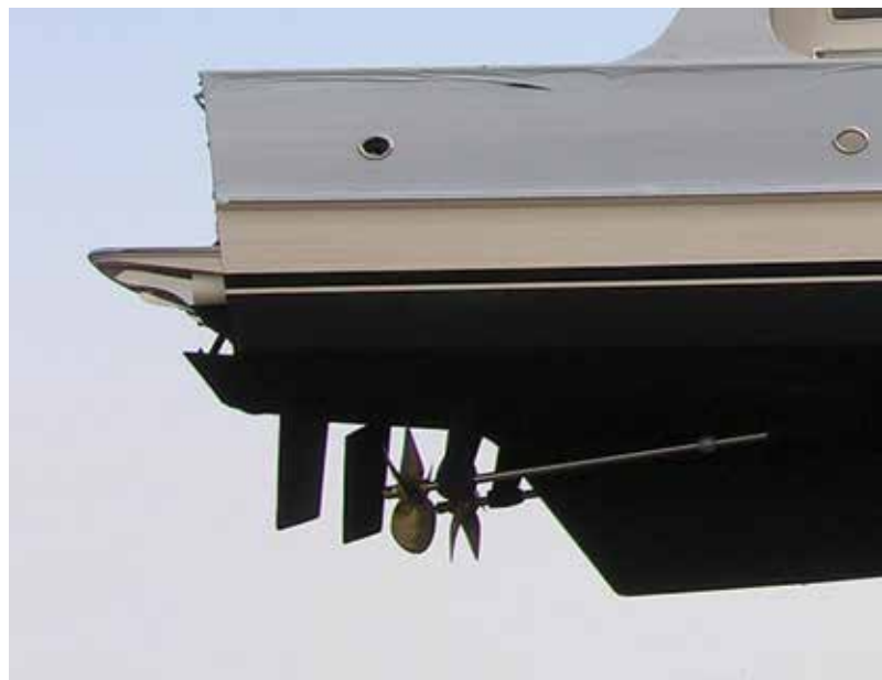
Deep full-length keel protects the running gear
