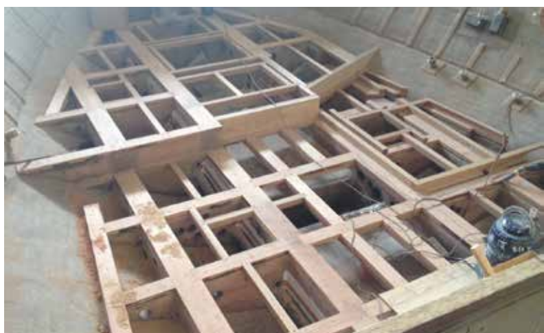
Hull reinforcement stiffens a solid glass hull
