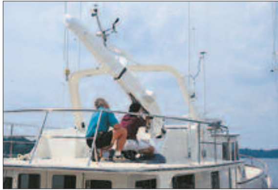
Pat Flaherty checks installation of davit system for handling dinghy.
