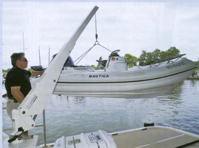
Ray Currey of Burr Yacht Sales demonstrates how easy it is to launch this yacht tender from the roof of a new Fleming 55 using a Steelhead hydraulic-davit system.
