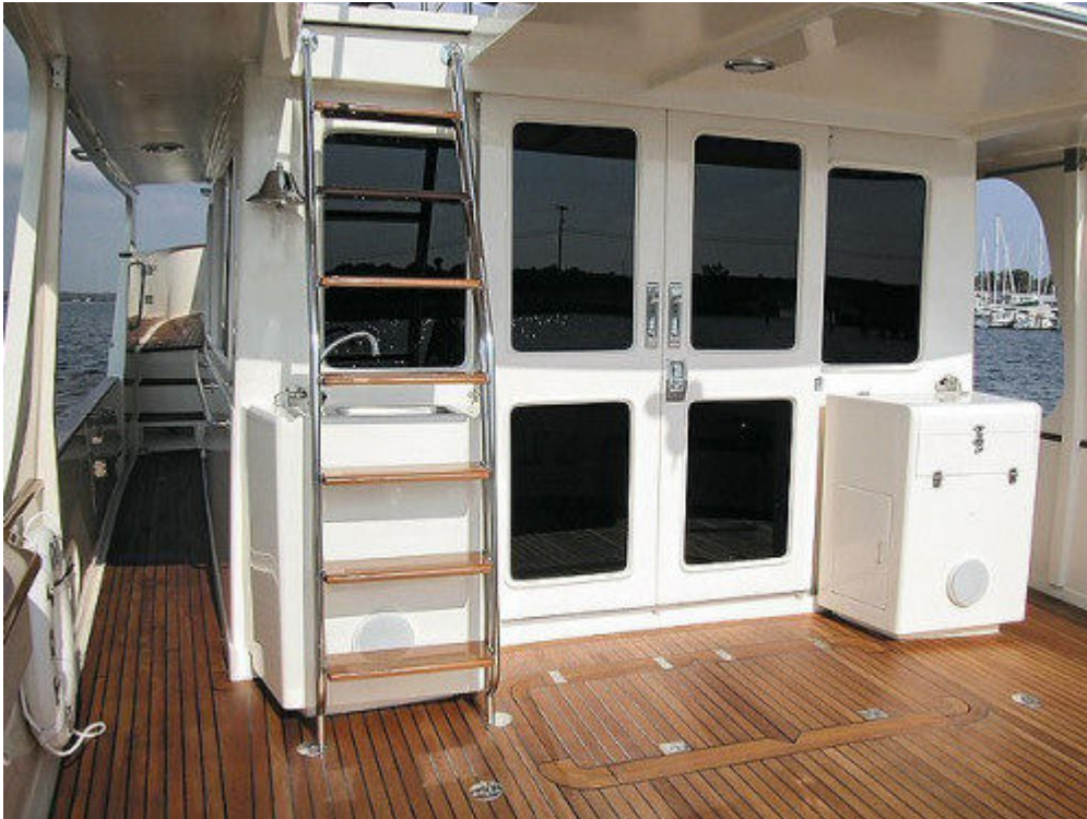
The aft doors are fiberglass and have "seadog"-style latches. The console to starboard is optional and can contain most anything an owner wants. The teak deck and the teak treads on the stainless steel ladder are all standard. The hatches in the deck lead to the lazarette.
