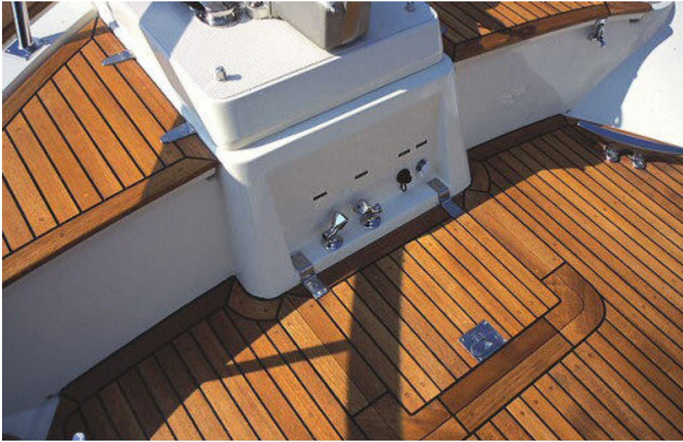
Here we see a standard teak and Thiokol deck. Note the freshwater and saltwater bibs for cleaning the ground tackle and deck.
