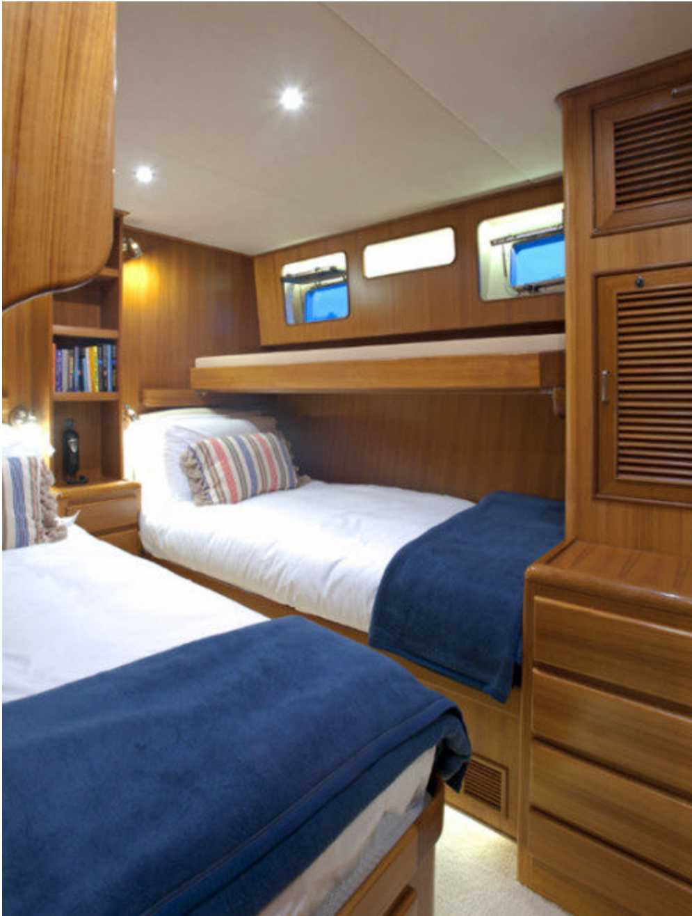
This is the VIP stateroom on the port side. Note the wood bulkheads, drawers and louvered doors. Instead of having a Pullman which can be problematic to raise and make, Fleming prefers the sliding bunk seen above which tucks under the side deck.
