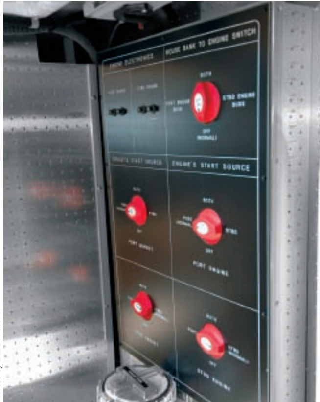
Top: My only nit on the new Fleming 55 is the use of non-marine Racor fuel filters, a frequent and common error on boats from the East. This yacht deserves the filtration offered by Racor's MA Series (Marine) fuel filters, which have USCG-approved stainless-steel shields, clear bowls, and metal drains. Above: The master battery disconnect switches are easily accessed in the main lazarette space, out of the engine room. This is the way all boats should be built, and this is as good as it gets.
