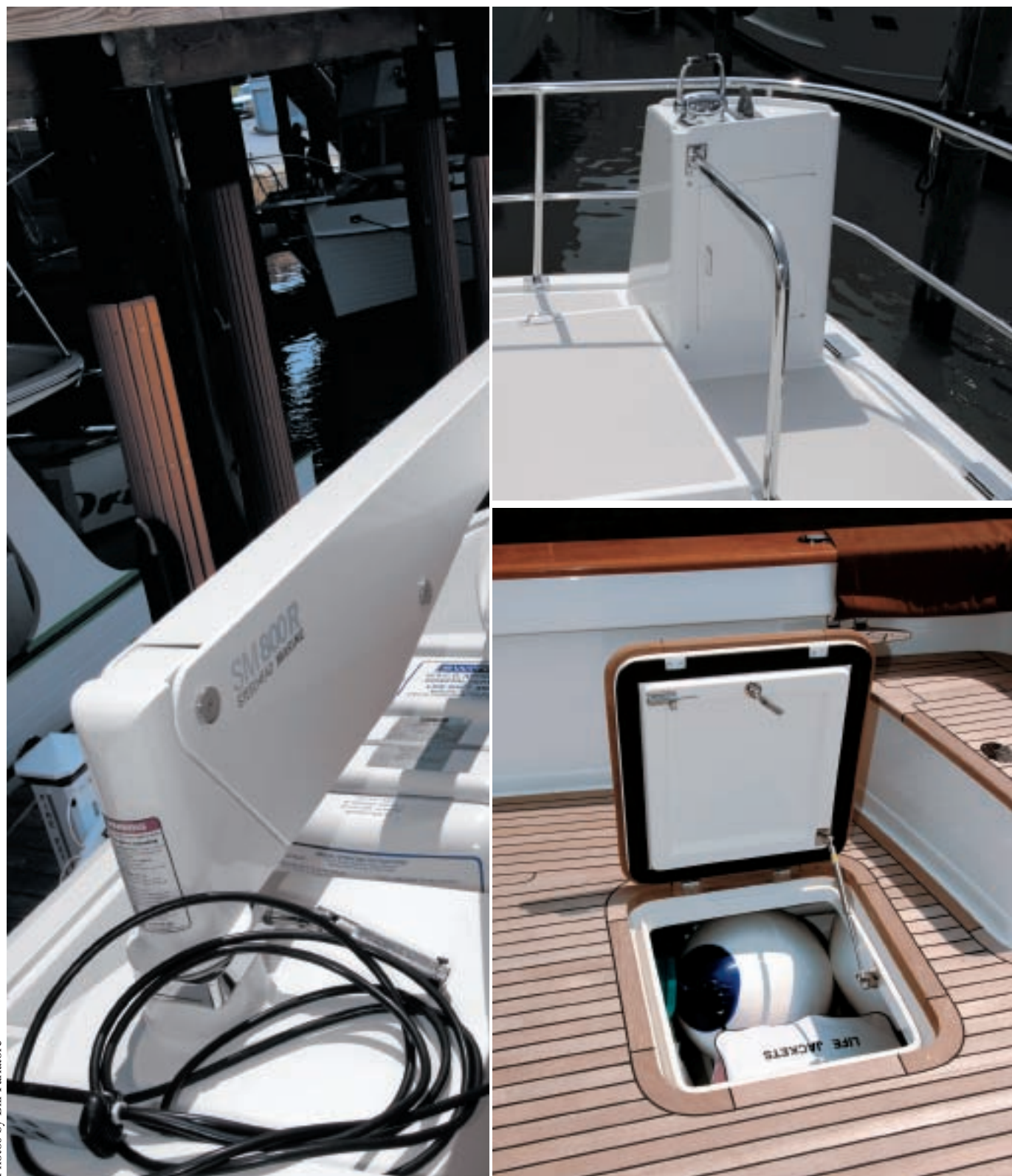
Left: The davit crane can lift the tender and place it over the side with complete control, as it can extend or retract to handle the balanced RIB without theatrics. Top right: The new control station option on the aft end of the boat deck provides great control while docking and has proven a popular choice for all of the latest boats. Above right: The gas strut holds the hatch open and the cavernous lazarette holds all the cruising gear and accessories one could imagine. Every detail of the hatch is thought out and done right. Very nice and consistent with the rest of this continually-improving cruising boat.
