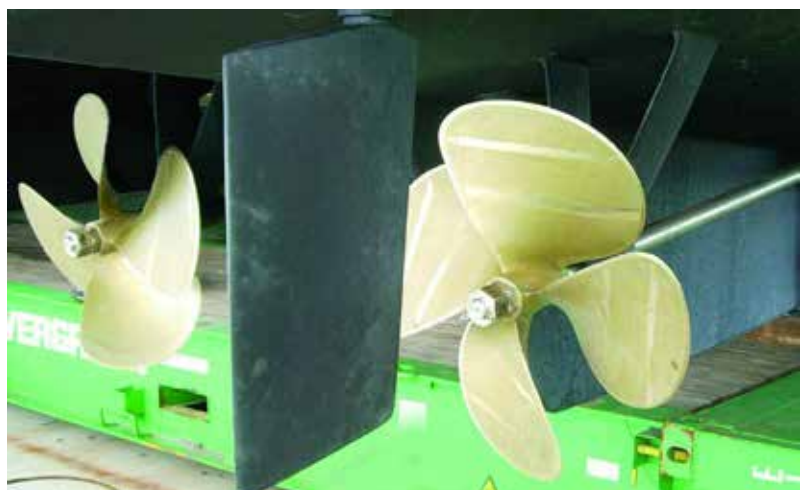
Deep full-length keel protects the running gear
