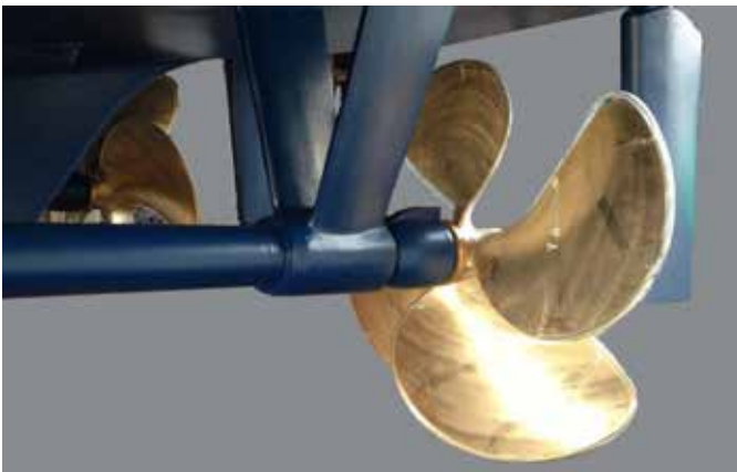
Seatorque shaft tube with rope cutter
