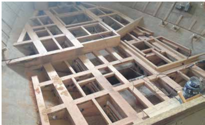
Hull reinforcement stiffens a solid glass hull
