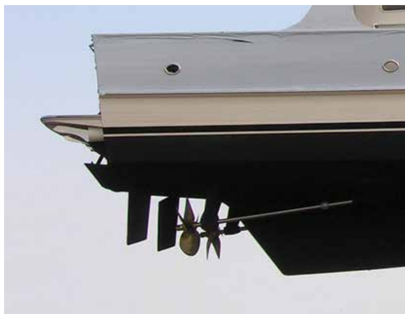
Deep full-length keel protects the running gear
